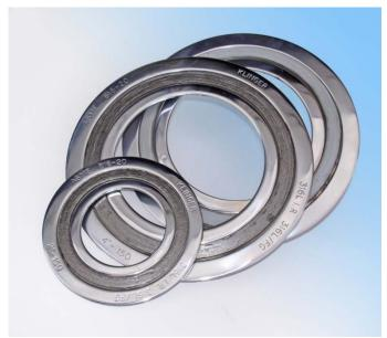
Maxiflex sealing element consists of a pre-formed metallic winding strip with layers of a softer, more compressible sealing material which, during compression, is densified and flows to fill imperfections in the flange surfaces when the gasket is seated. The metal strip holds the filler giving the gasket mechanical resistance and resilience.
